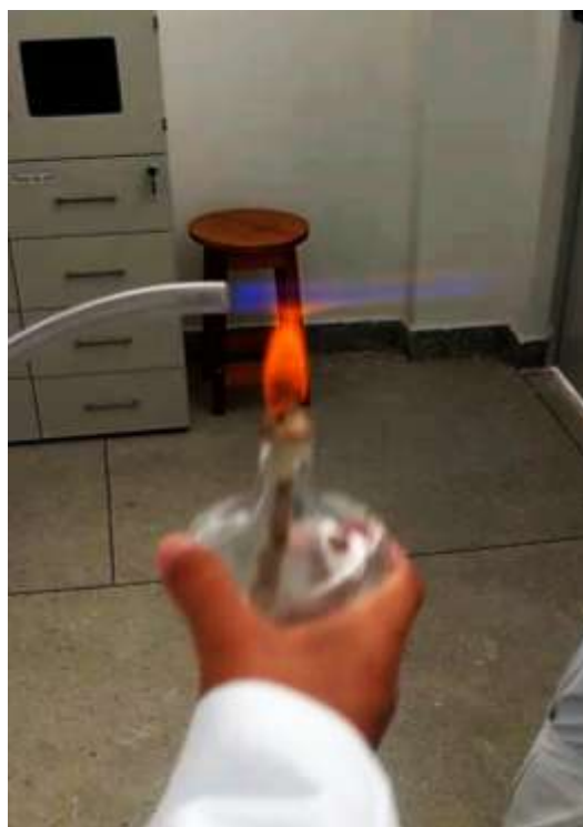
Figure 5 – Burning of the gas obtained from biodigester.
